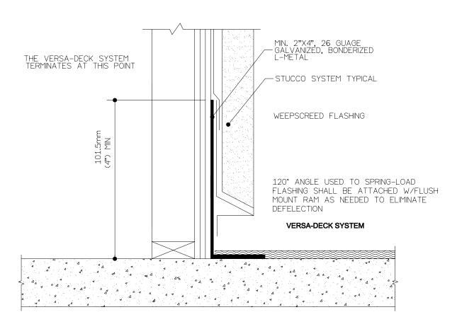
CONCRETE SUBSTRATE 1/8" SLOPE PER FOOT
