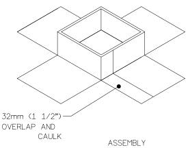
FACE NAIL (A MIN. OF APPLY MANUFACTURER RECOMMONDED JOINT SEALANT BEHIND FLASHING AND AT THE TOP OF THE FLASHING. TWO NAILS PER SIDE) AT THE FLASHING ON EACH SIDE OF POST 11111 1111114 FLASHING IS SECURED -TO SUBFLOOR WITH NAILS ON ALL SIDES APPLY MANUFACTURER RECOMMENDED JOINT SEALANT AFTER COMPLETION OF THE VERSA-DECK SYSTEM AROUND BASE OF POST. VERSA-DECK SYSTEM TERMINATES AT THIS POINT GALVANIZED, 26 GUAGE, FLAT METAL INSTALLED ON ALL CORNERS OF THE
