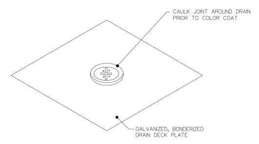
DRAIN DECK PLATE MEASURES 230mm (9") SQUARE FOR 50mm (2") DRAIN 250mm (10") SQUARE FOR 76mm (3") DRAIN
